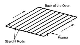
To remove a shelf slide the shelf towards you until the shelf stop is reached. Tilt shelf up at the front so that the stops clear the side supports. Lift shelf clear. To install a shelf, reverse the above steps. Each shelf position has an upper and lower support wire. ensure the shelf is placed between these two support wires.
